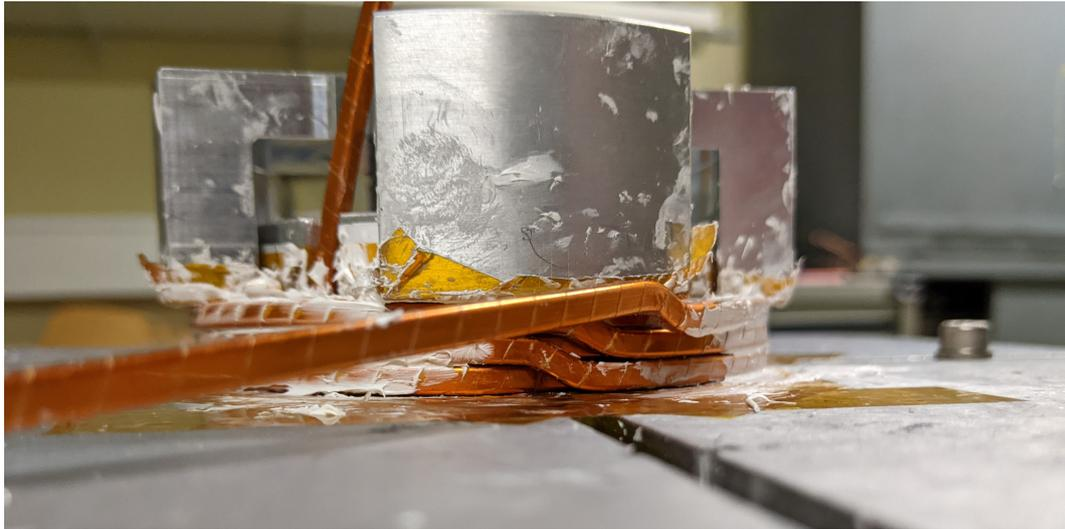
**Figure A.2:** The coil is wound around an aluminium cylinder. A stamp is used to ensure that the height of the coil is up to specifications. Before the coil is wound around the cylinder the wire is pre-bend. In the image it is shown how these bends line up in order to allow the wire to transition to the next layer.
