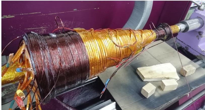
Figure 5-12: Finished Zeeman slower clamped in the lathe. The three different parts are well distinguishable.
