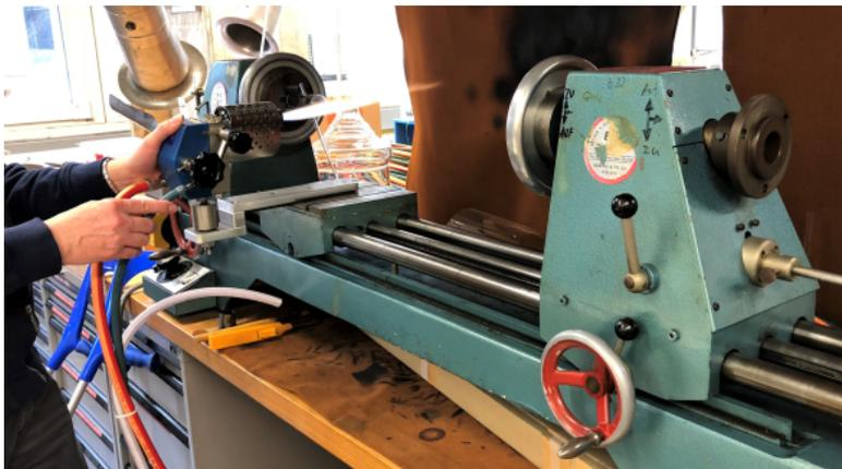
Figure 4.11: The glass-working lathe used in the glass workshop of the university. The burner softens the glass while it is rotated. This allows a symmetrical work on the cylindrical glass tubes.
