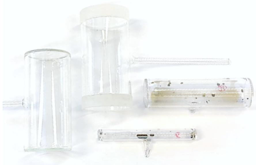
Figure 4.12: Design of various cells. The two cells on the right are already closed and filled with caesium.
