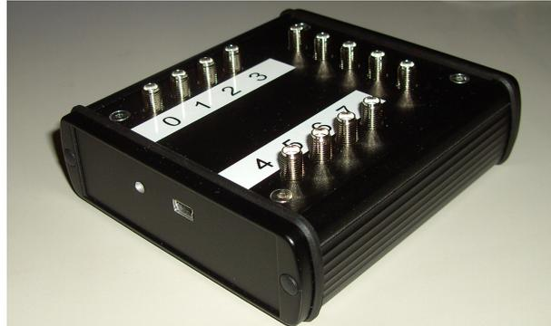
Figure 3.7: FPGA based Time-Tagger with 8 independent channels for time-resolved counting of digital pulses
