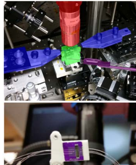
Figure 2. (top) Optical setup for device characterization. (bottom) A chip with multiple cavities addressed by optical fibers. [Courtesy of: A. McClung, PhD thesis, Caltech, June 2017].
